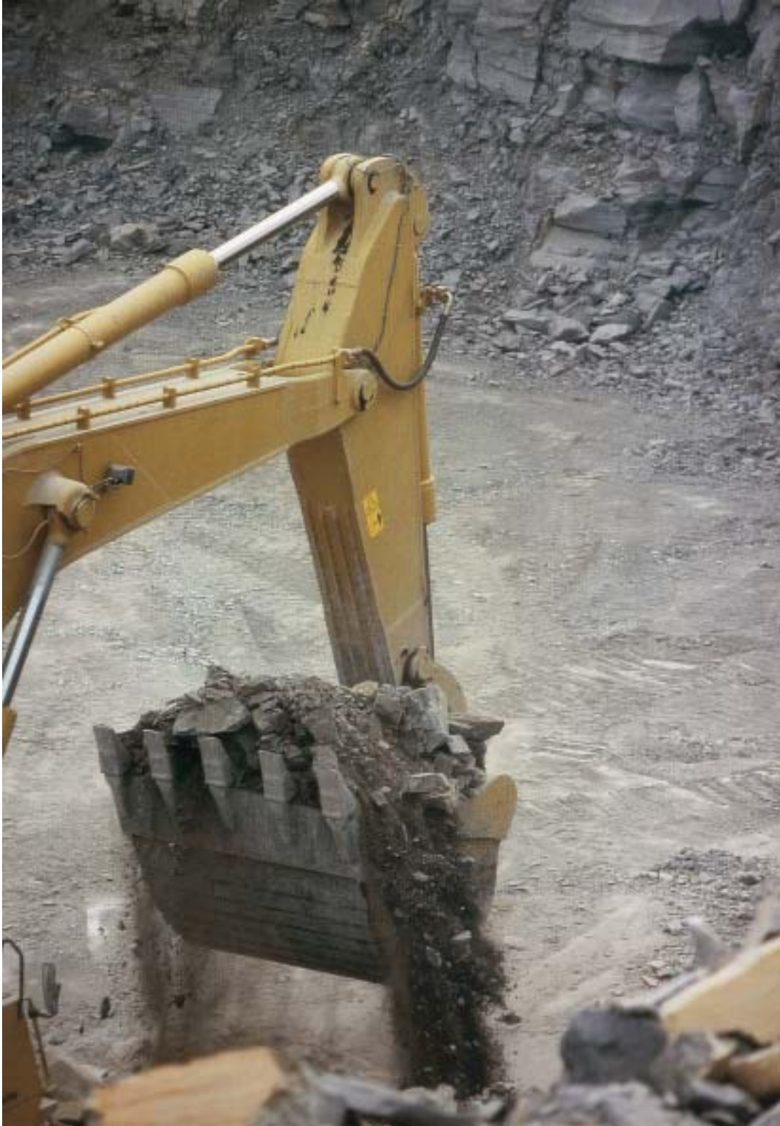
Figure 1: Excavator shovel made of DILLIDUR-V steels in the harsh conditions of open-cast mining (Illustration used with the kind permission of Schlüter Baumaschinen, Erwitte, Westphalia, Germany)
