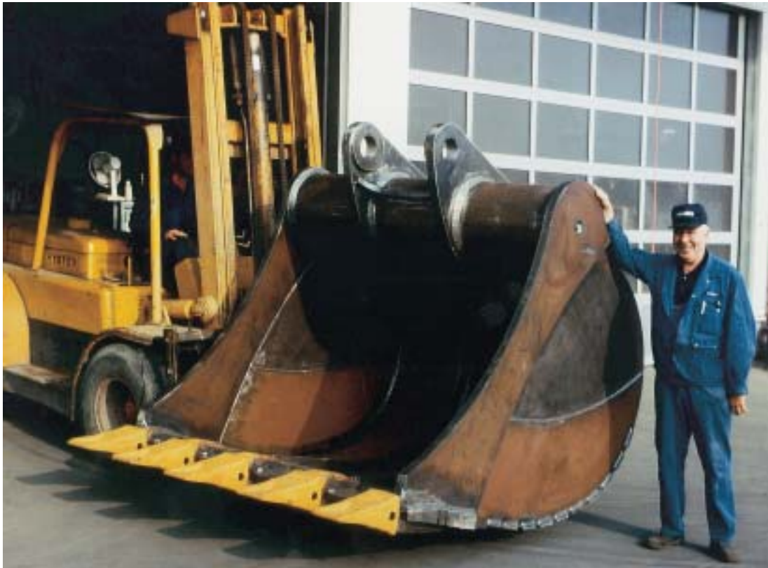
Figure 20: Welded excavator shovel made of DILLIDUR V plates (Illustration used with the kind permission of Schlüter Baumaschinen, Erwitte, Westphalia, Germany)
