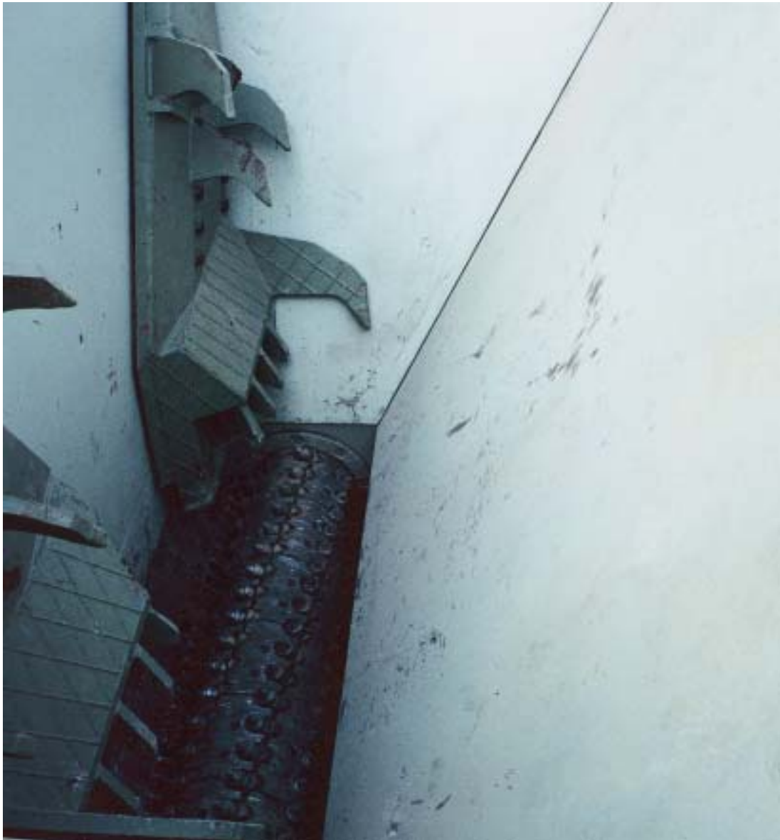
Figure 6: Charging hopper of a crushing plant, walls made of DILLIDUR 400 V
