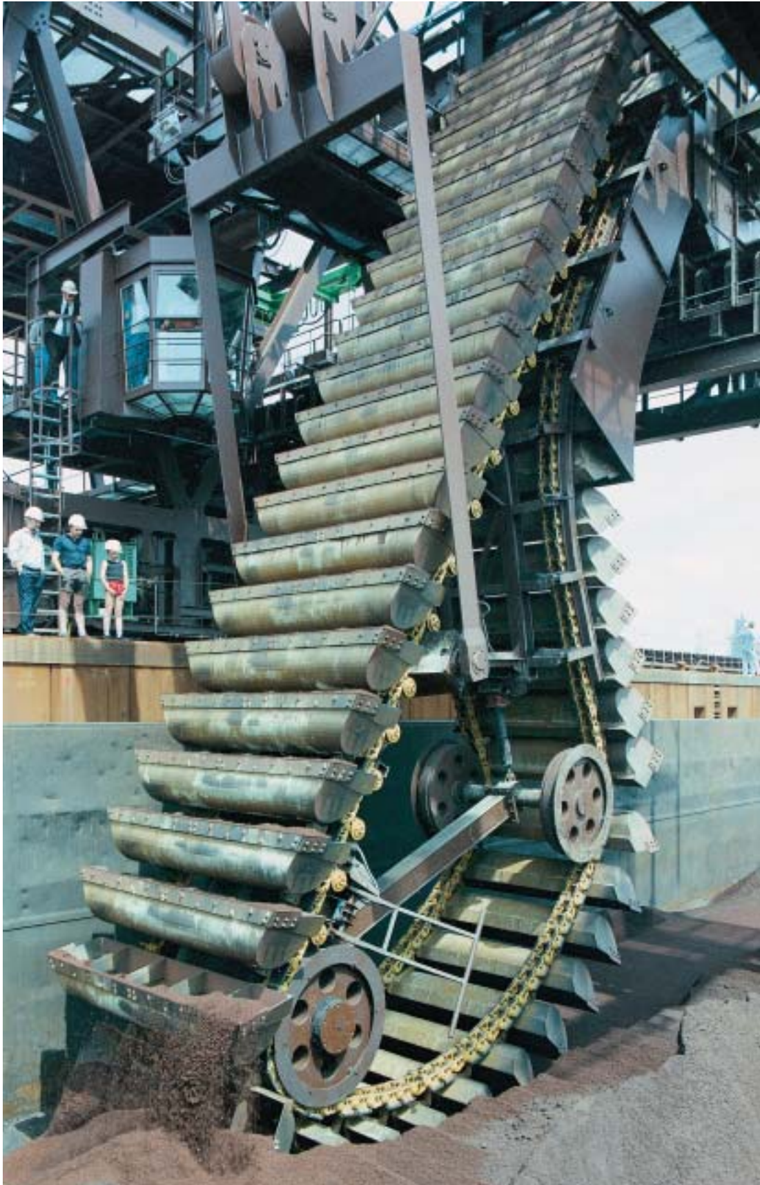
Figure 10: Continuous ship unloader in the harbour of DILLINGER HÜTTE GTS
